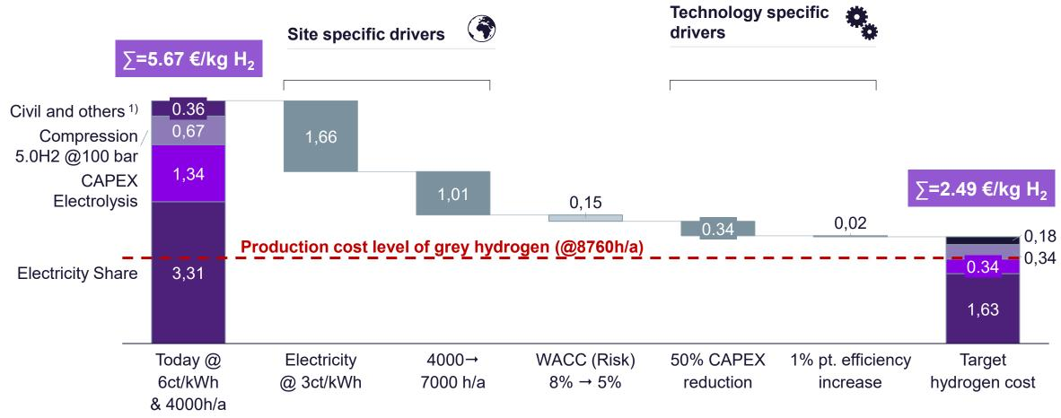
Note: Electrolyzer power: 55  $Mw_{el}$  (72 modules); Hydrogen production: 1005 kg/h (H5.0 @ 100 bar) with 99.999% purity
